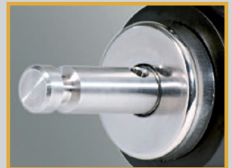
Stainless Steel protection caps secure the seals from fishing lines.
