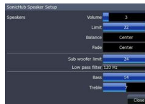
Speaker adjustment screen showing Sub Woofer bandpass control
