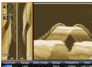
Submerged bridge in 30' of water with handrails clearly defined - almost photographic.
