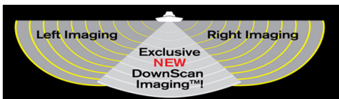
How it works: SideScan left and right, and DownScan Imaging™ below
