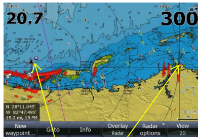
Broadband 3G seeing Tarpon Spring Power Plant Stack at >15nm away
