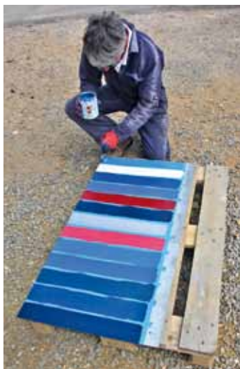
We immersed a static test panel of the 12 antifoul paints into the West Solent
